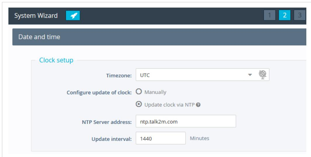
Fig. 2 NTP Settings in the Flexy System Wizard
