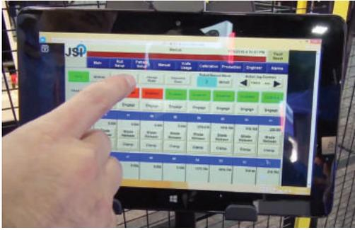
The same view. With the help of eWON Cosy, operators can view the same thing on a tablet or smartphone as they would on the machine HMI, allowing for remote access inside the plant or indeed, anywhere in the world
