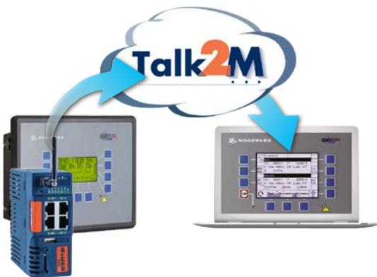
The eWON Cosy is connected to the Woodward PLCs and HMI. The Cosy establishes a secure tunnel via the Talk2M cloud service. By logging on to Talk2M, it is possible to configure and commission the gensets. Just as if connected on site.
